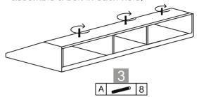
Assemble one bolt in each hole in the armrest.
